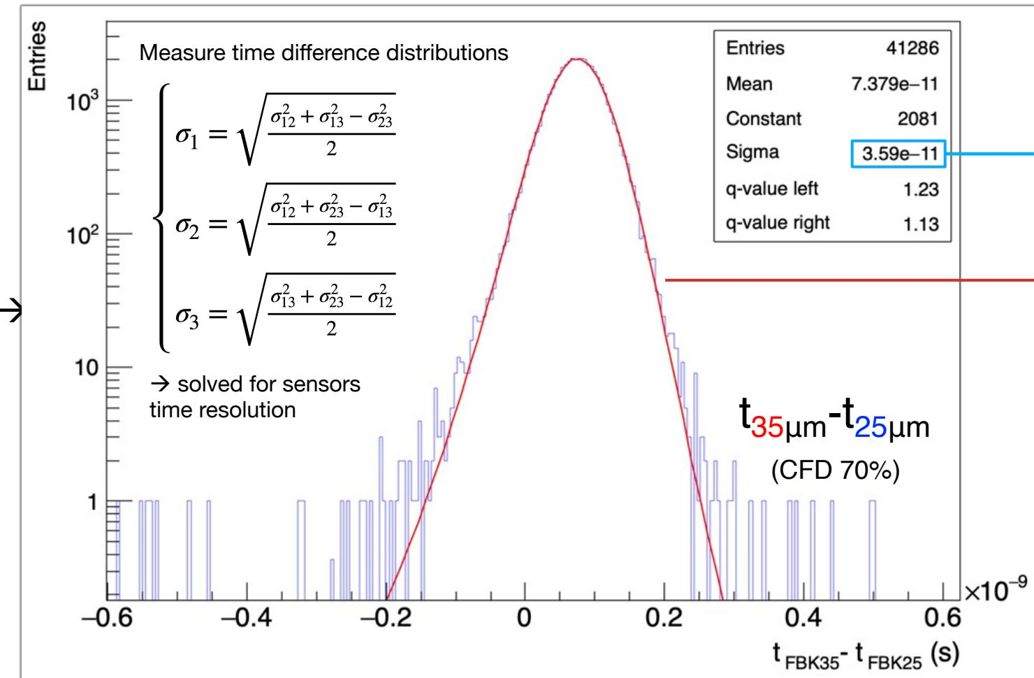
Measurements in full bandwidth (4 GHz) → Smoothing to remove high frequency noise → 1 GHz
