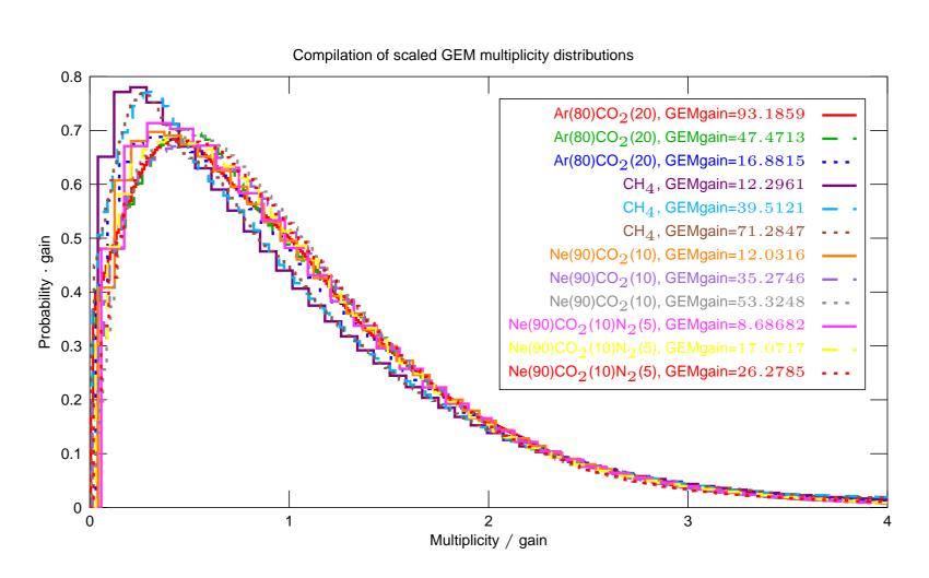
Preliminary results show that shape of GEM avalanche response distribution is approximately independent of the effective gain, and slightly depends on the working gas (better for Neon based).
