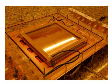
Front-End Electronics and LED electronics from the Leopard project (NIM **A694** 16, POS **TIPP2014** 056).
