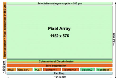
Schematic view of architecture of Mimosa-26 chip
