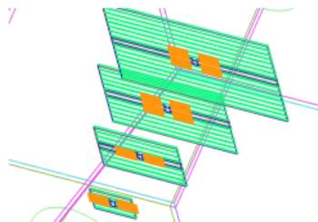
Layout of prototype vertex detector with sensor locations shown as orange boxes
