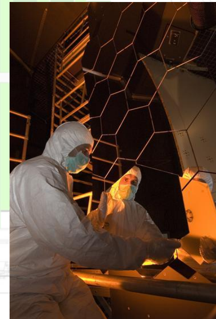
Assembling RICH 2; note the mirrors
