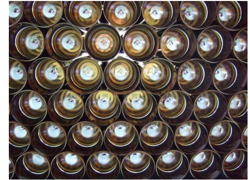
Array of RICH photodetectors
