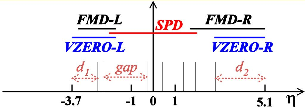
Left-side 1-arm trigger : no signal with  $\eta > +1$
